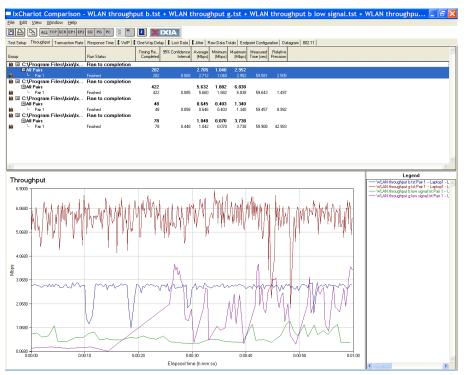
**Figure 3a**. Compares the performance of 802.11b and 802.11g (only) test using standard IxChariot long connection script Filesndl
