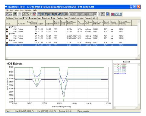
Figure 4c. MOS measurement for VoIP traffic with different codecs
