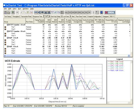
Figure 4b. MOS score drops to 2.06 with the addition of data traffic
